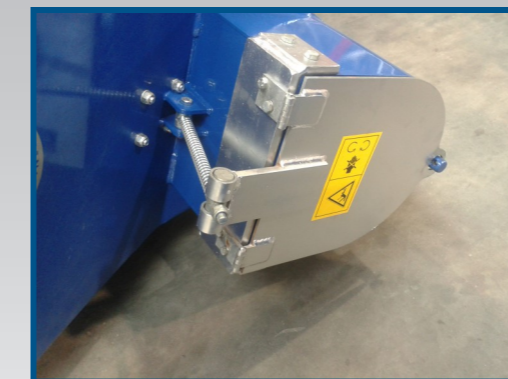
mechanical shut-off valve
