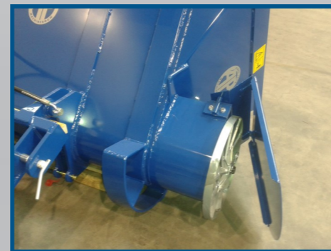
fodder beet cutting device VDCE (8-bladed knife)
