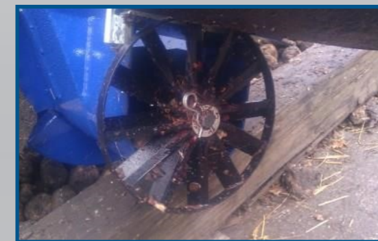
fodder beet cutting device with potato knife (10-bladed)
