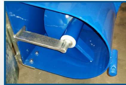
low-maintenance auger suspension
