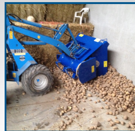
one-sided discharge, equipped with potato cutting device
